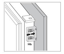
14. Press the part (Hd) on the part (Hb). Do a final check to make sure that:
